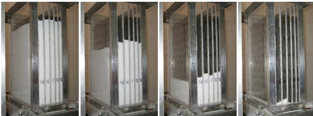
Fig.4 – Flowability test at different times
