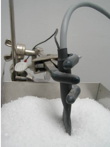
Fig.1 - Thermal Conductivity test
