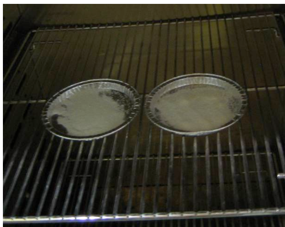
Fig. B3 – Oven test for Moisture Content
