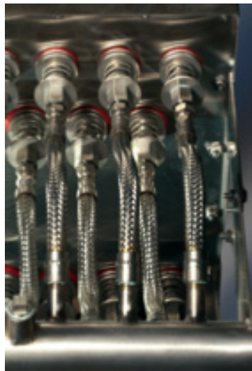
Figure 6 - Individual connections from plate to manifold
